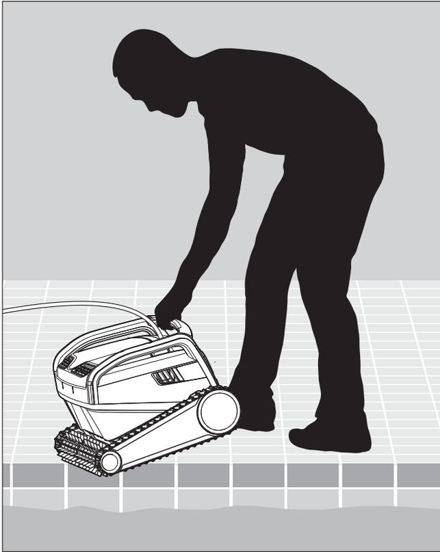
**5.2.1** Place the Robotic Pool Cleaner in the pool. Release it and let it sink to the floor of the pool. Make sure that the floating cable is free of any obstacles.
